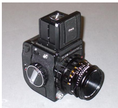
The Kowa Super 66 Medium Format Single Lens Reflex Camera and Removable Back from 1975
